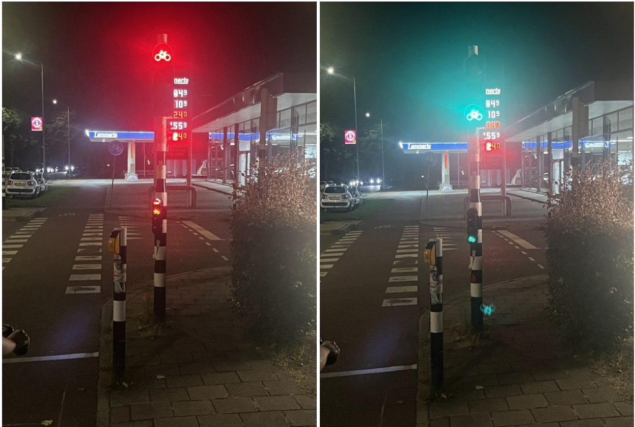
Figure 9. Loop in cycleway priority activated cycling green light. Time counter how long still on red. Nijmegen, Netherlands.
